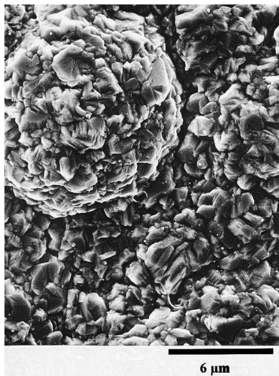
Fig. 8. SEM observation of electrodeposited copper in 1 M \text{CuSO}_4 + 0.1 M \text{H}_2\text{SO}_4 solution under following conditions: duty cycle 2/2.2, current density 1000 \text{ A m}^{-2} and deposition duration of 3600 s.
